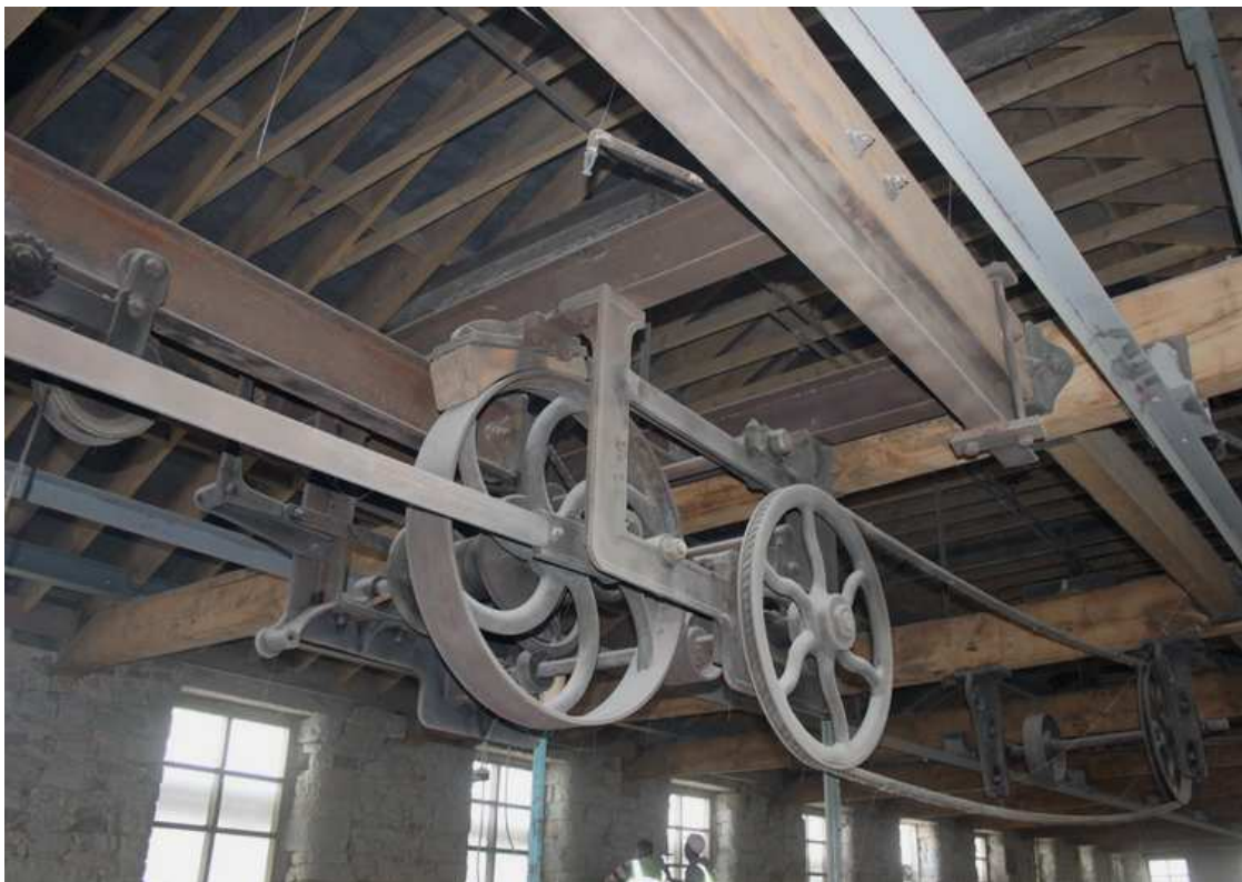
Plate 39: Original hoist on third floor of spinning block
